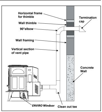
Figure 12: Vertical rise with Horizontal Termination.
